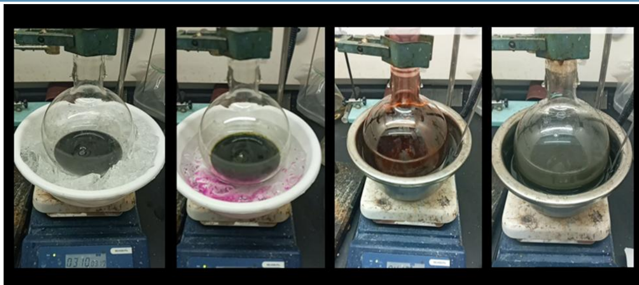
Figure 1. Photographs describing the preparation process of GO by Tour's method: (A) before addition of potassium permanganate; (B) after oxidation; (C) after pouring on ice; (D) after addition of H_2O_2 .
